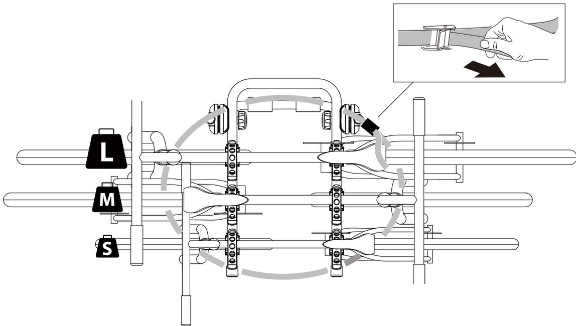
GB-US - Double check that all the straps are correctly tightened after installing the bikes
